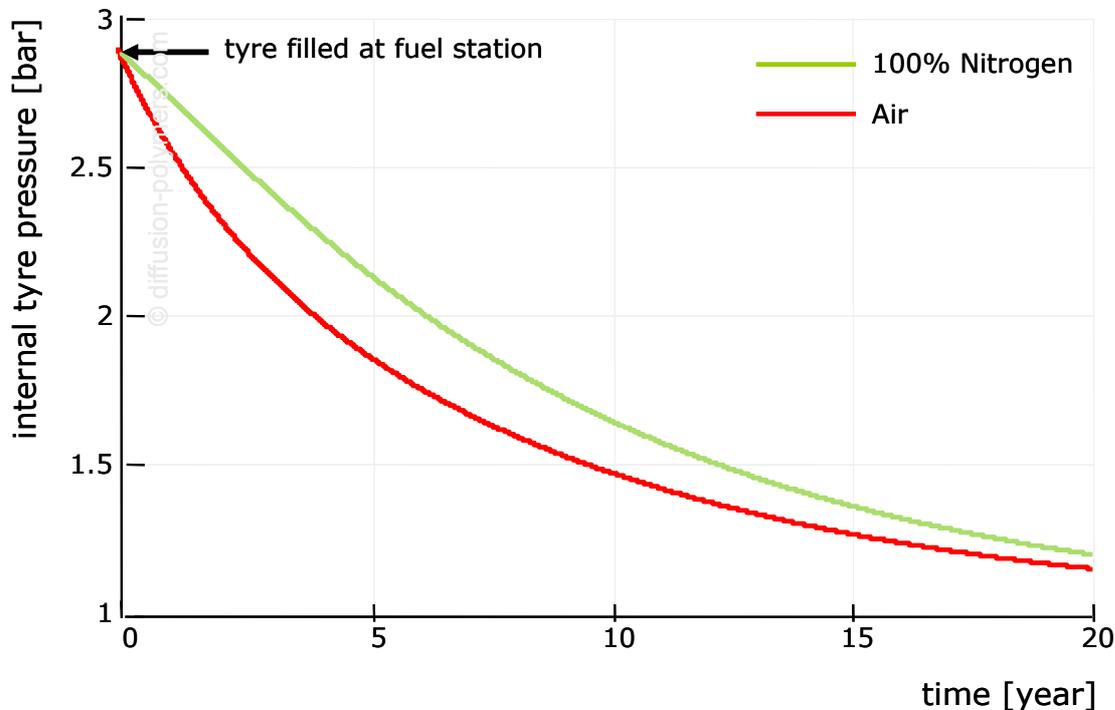
From the graph it becomes obvious that the internal pressure drop in the tyre goes slower if the tyre is filled with 100% Nitrogen. The difference during the first years is 40%. Tyres are usually refilled after 0 to 15% loss of pressure, so we may assume that during normal operation the advantage is a stationary 40%.
