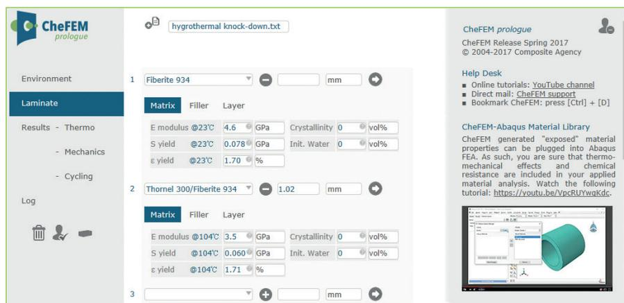
Fig. 1: The CheFEM user interface, with unexposed pristine Fiberite 934 defined in layer 1, and exposed filled Fiberite 934 defined in layer 2
